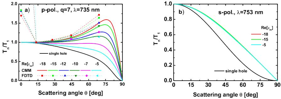
**Figure 3.4:** Distribution of the transmitted power as a function of angle for different values of  $\text{Re}(\epsilon_m)$ , calculated with both CMM model and FDTD; for the latter we show  $T_n/T_1$ , transmission per diffraction order normalized by the first diffraction order. Panel (a) is for p-polarization, while panel (b) renders the results for s-polarization.
