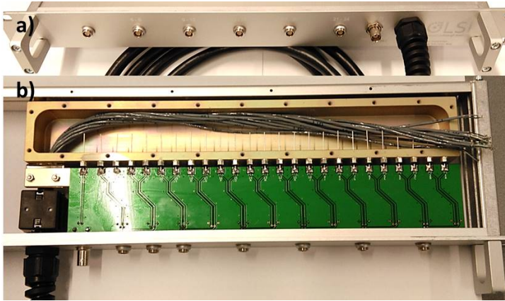
Figure 6.12: Breakout box as manufactured by LSI B.V. a) front panel with 6 \times 4 -pins LEMO connectors. b) Inside of the breakout box. The cabling inside the RF-shielded box have yet to be connected to the EMI feedthrough filters. This box has a frontpanel with 5 \times 4 - and 2 \times 2 -pins LEMO connectors. The single BNC connector, which is connected to the inside shielding of the black cable, can be used to measure noisy voltages between cryostat and 19" rack.
