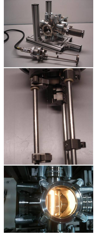
Figure 6.6: top : anneal-o-tron, middle : clamps holding a 25\ \mu\text{m} diameter wire, bottom : annealing of niobium wire.
