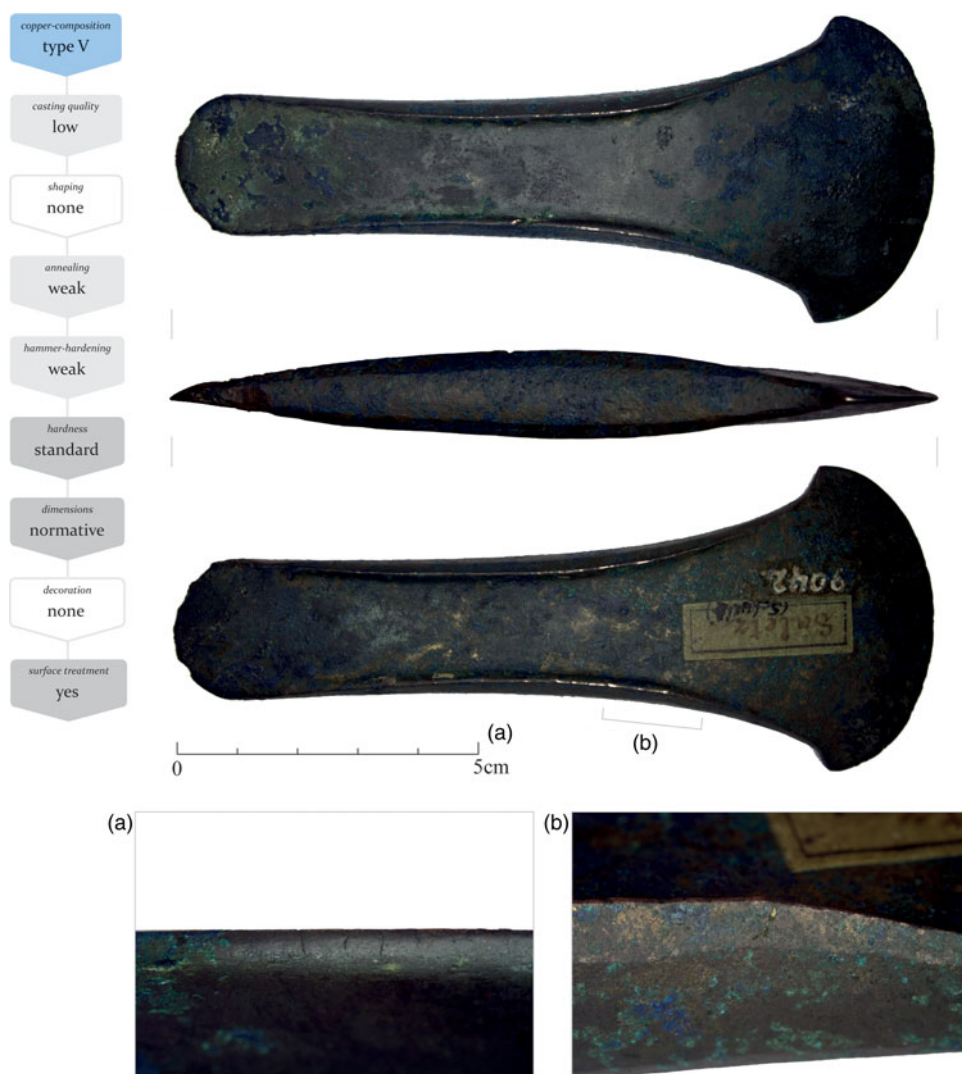
Figure 6. Left: Chaîne opératoire of axe 3. Right: Axe 3, a type Salez from Sennwald-Salez in Switzerland, a hoard find. Note the starting cracks (a) in the flange. Photographs by the author, courtesy of the University of Vienna.
