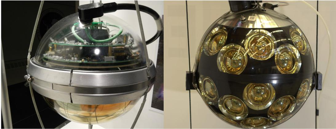
Figure 2: A picture of an IceCube module (left) and a KM<sub>3</sub>NeT module (right), showing the difference in light sensors.
