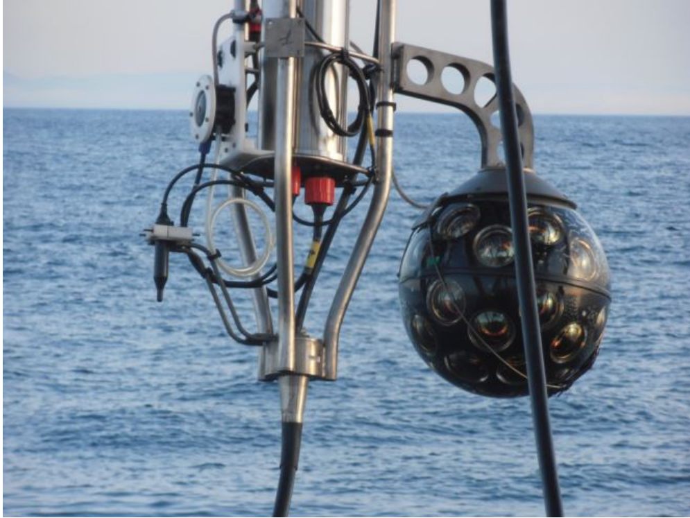
Figure 23: The PPM-DOM attached to the ANTARES instrumentation line before deployment.
