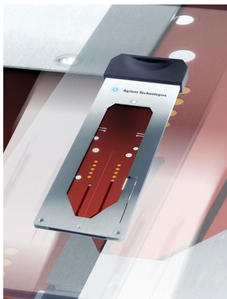
Figure 6 | Agilent LC-MS Chip™. 33
