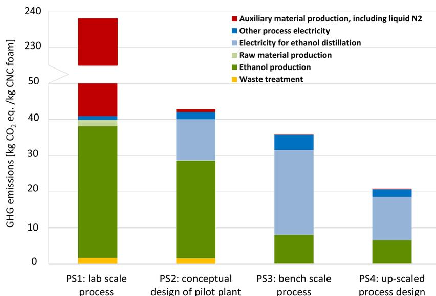
Fig. 4. Cradle-to-factory gate GHG emissions of 1 kg CNC foam at four R&D stages.
