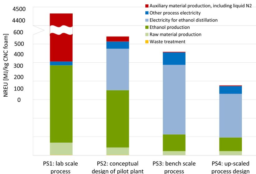
Fig. 3. Cradle-to-factory gate NREU of 1 kg CNC foam at four R&D stages.
