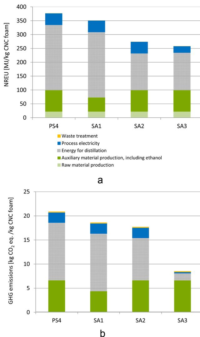
**Fig. 6.** Results from sensitivity analyses for a) NREU and b) GHG emissions for producing 1 kg CNC foam. Please refer to Table 3 for the three cases of the sensitivity analyses.
