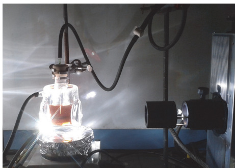
Figure AI.2. Irradiation setup for a preparative scale photoreaction under Ar.
