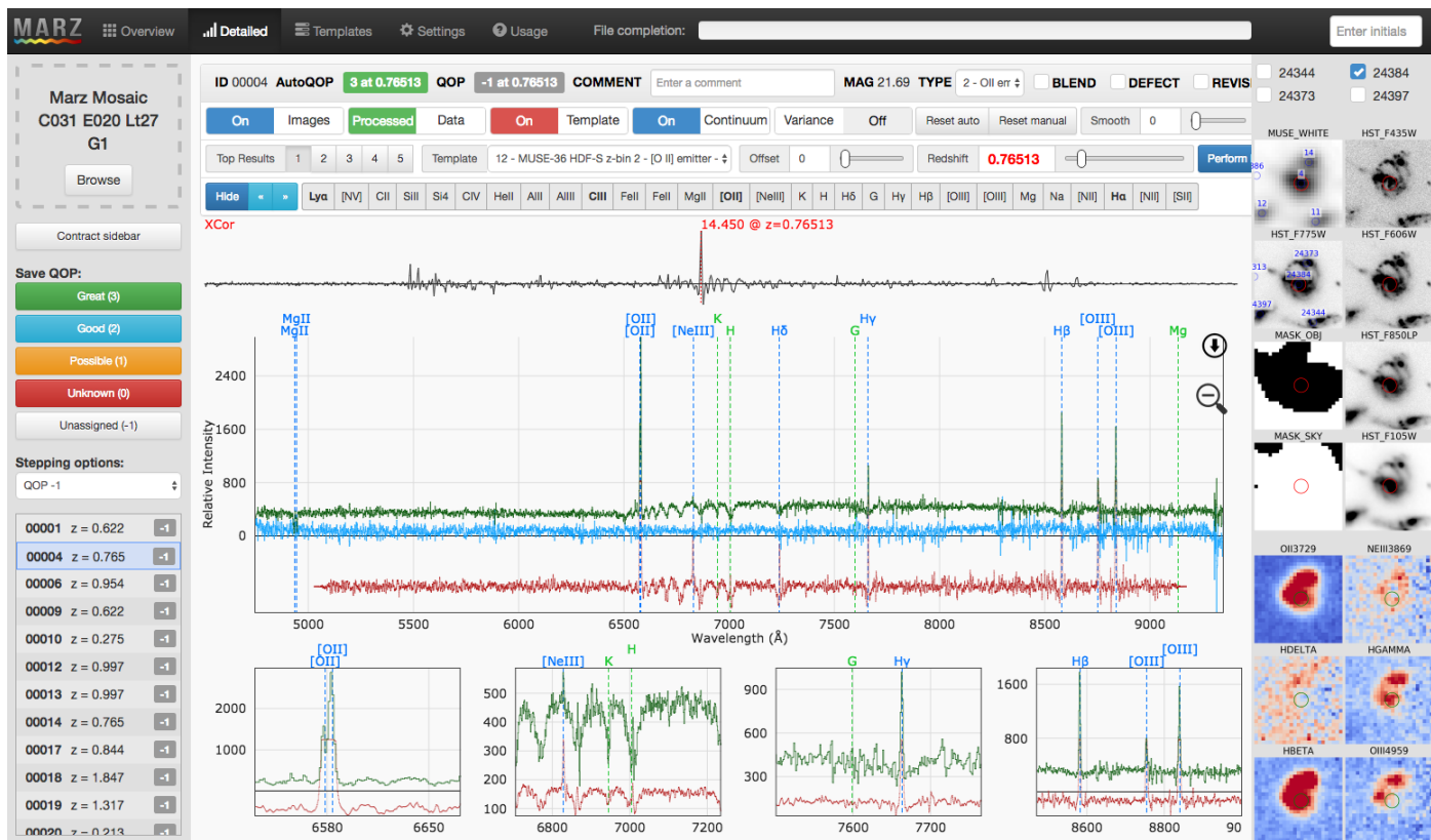
Fig. 1. Redshift tool MARZ with some modifications for our redshift analysis. This tool reports the most likely redshift and the quality (QOP) by cross-correlating with input spectral templates. The redshift identifiers verify the suggested redshift or manually find a better redshift and provide its quality (indicated as CONFID in the catalogs). We also implement a feature to show images in the panel on the right.
