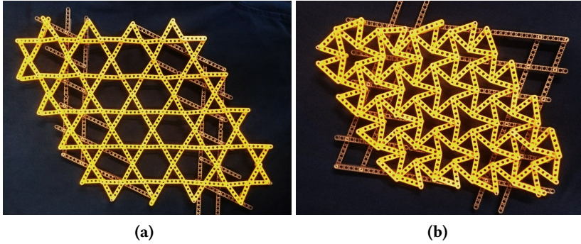
Figure 1.1. Model of a mechanical metamaterial: twisted kagome lattice. As all the small triangles twist together, the whole structure in (a) contracts to the one in (b).
