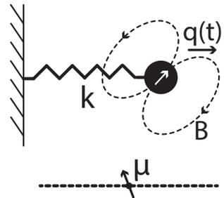
Figure 3.1: Schematic representation of spin  $\mu$  interacting with a mechanical resonator with spring constant  $k$  and displacement  $q(t)$  of the magnet. The dashed line shows the position axis that is used in Fig.3.2.
