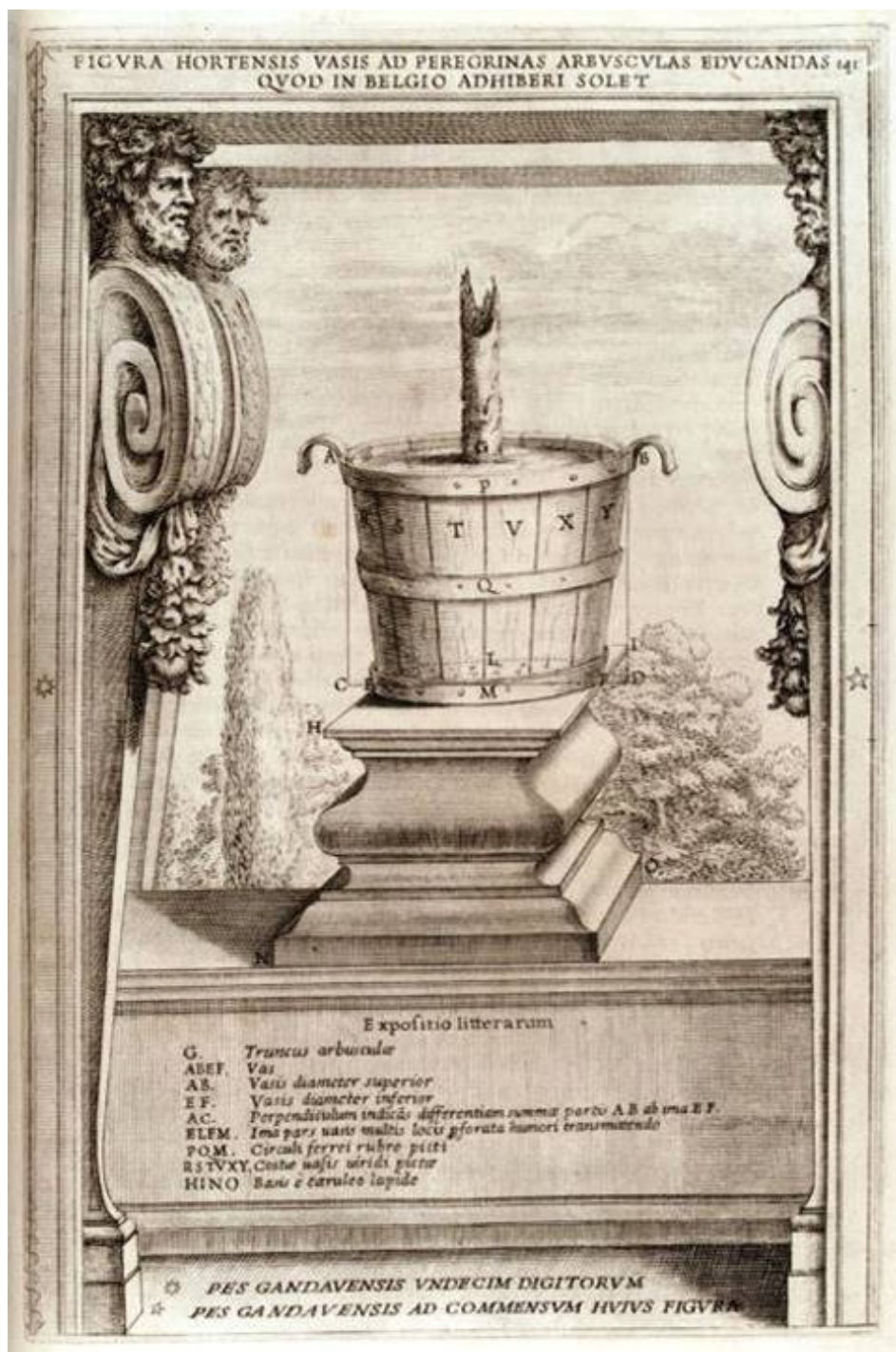
Figure 67: Willem de Blasere's invention of a tub for orange trees. From Ferrari.
