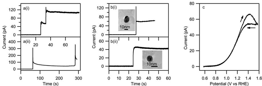
Figure 5.4: (a) AuNPs landing on a carbon coated Cu TEM grid (at 1.25 V) in presence of  $\text{N}_2\text{H}_4$ . (b) Landing events of individual AuNPs, with the same AuNP imaged by TEM afterwards. (c) CV ( $200 \text{ mV s}^{-1}$ ) measured at the individual AuNP shown in (b(i)).
