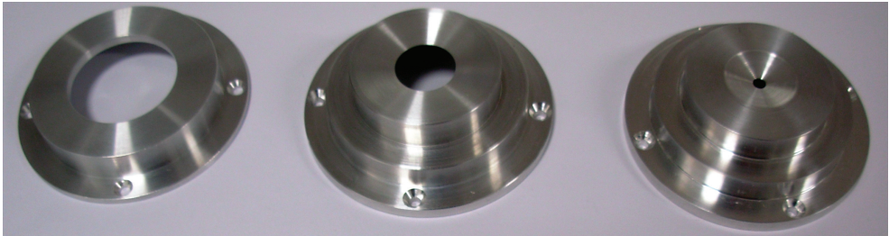
Figure A.4: Different radiation heat shield designs improving the final cooldown temperature of the sample from 12K (left) to 7 – 8K (center) to 4.8K (right).
