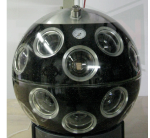
Figure 12.1: The prototype of the KM 3 NeT digital optical module (DOM). Credit: Proprietary KM 3 NeT Consortium, http://km3net.org
