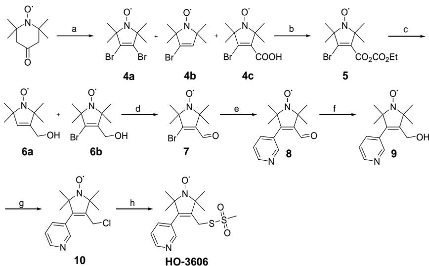
**Scheme 2.** Synthesis of HO-3606. (a) NaOBr, water/1,4-dioxane; (b) ClCO<sub>2</sub>Et, Et<sub>3</sub>N, Et<sub>2</sub>O, 0 °C to RT, 3 h; (c) NaBH<sub>4</sub>, EtOH, 0 °C, 4 h; (d) CrO<sub>3</sub>, pyridine, 0 °C, 30 mins; (e) Pd(PPh<sub>3</sub>)<sub>4</sub>, dioxane, 3-pyridineboronic acid; (f) NaBH<sub>4</sub>, EtOH, 0 °C, 4 h; (g) i) MsCl, CH<sub>2</sub>Cl<sub>2</sub>, 0 °C; ii) LiCl, acetone; (h) NaSSO<sub>2</sub>CH<sub>3</sub>, acetone/water, 40 °C.
