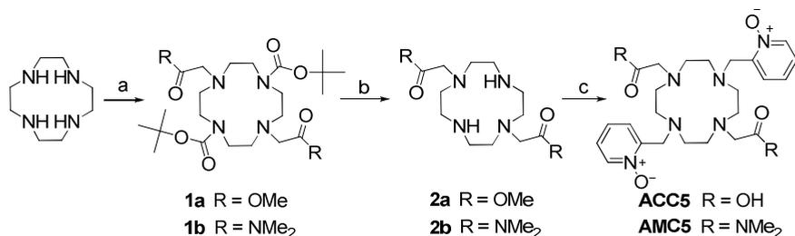
**Scheme 1.** Synthesis of AMC5. (a) i) BocOSu, CHCl<sub>3</sub>, RT, 1 day; ii) methyl bromoacetate or 2-chloro-*N,N*-dimethylacetamide, K<sub>2</sub>CO<sub>3</sub>, MeCN, RT, 16 h; (b) TFA, CH<sub>2</sub>Cl<sub>2</sub>, RT, 4 h; (c) K<sub>2</sub>CO<sub>3</sub>, 2-(chloromethyl)pyridine-*N*-oxide, MeCN, 80 °C, 12 h.
