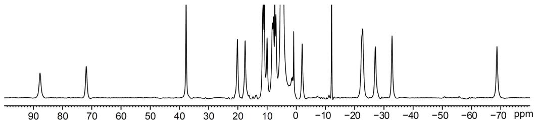
**Figure 6.**  $^1\text{H}$  NMR spectra of Yb-CLaNP-5-OMe complex.
