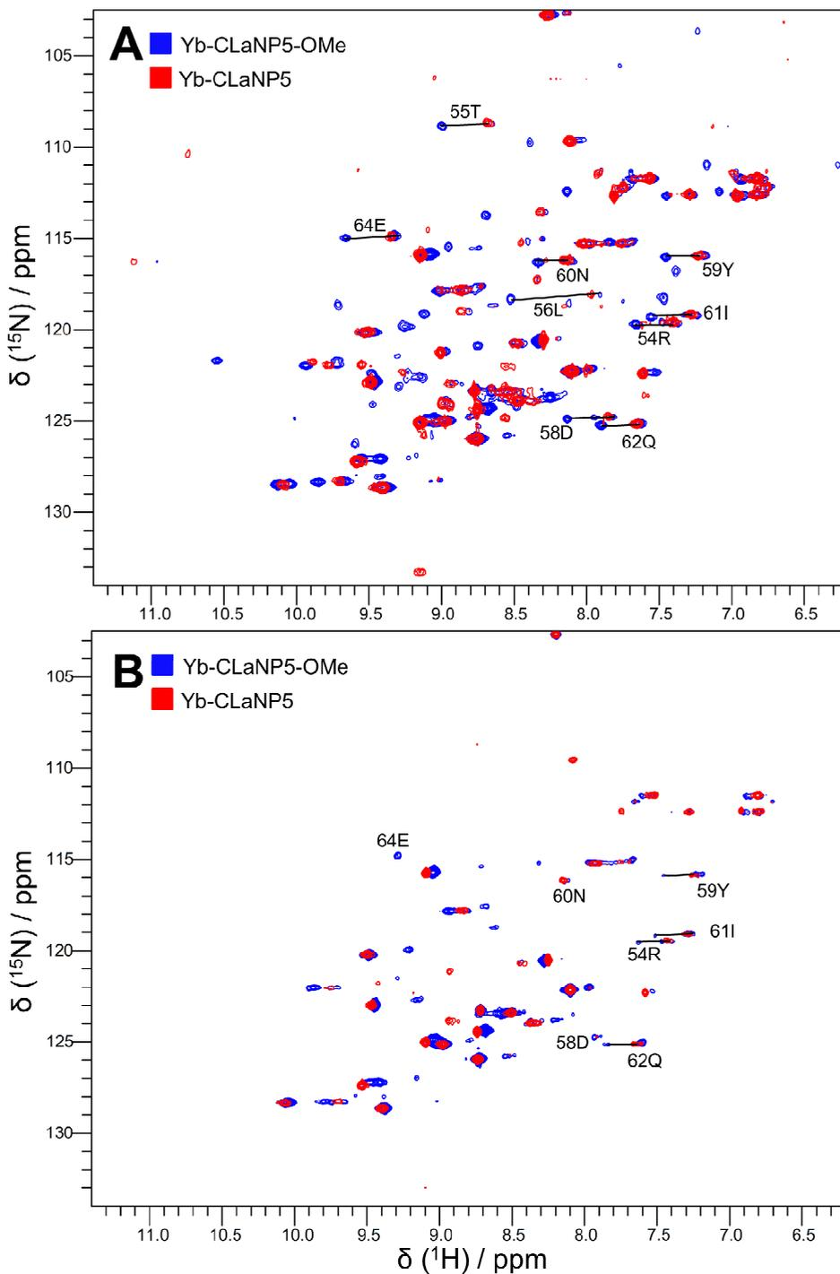
**Figure 3.** Overlay of  $^{15}\text{N}$ ,  $^1\text{H}$ -HSQC spectra of Ub A28C/D32C attached to Yb-CLaNP5-OMe (blue) and Yb-CLaNP5 (red) at 296 K (A) and 306 K (B). The assignment of amide proton resonances is indicated in solid line.
