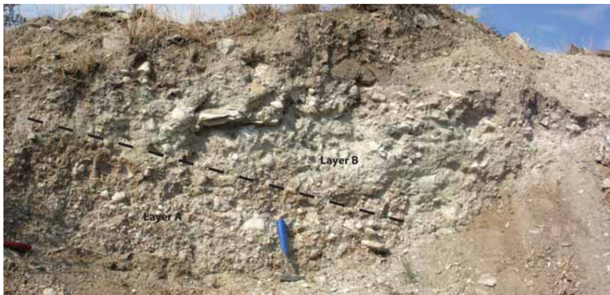
Fig. 4.24 Exposed profile at FS 30. The dashed line shows the approximate position of the boundary between the two layers. 'Layer B' is overlain by recent debris from construction works
