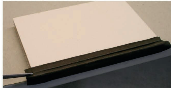
Fig. 211. The making of a partial leather binding. After the application of the spine leather, the extending leather at head and tail need to be cut in line with the joint, to allow for the making of the turn-ins.
