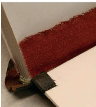
Fig. 212. Detail, after the cut was made and the small part of the spine leather was turned-in over the board edge.
