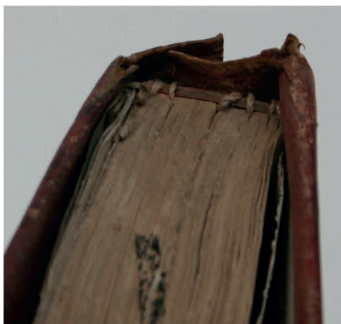
Fig. 195. UBL 891 E 37 (Singapore 1877). The endband core is a wooden stick, the secondary endband is missing.
