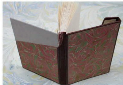
Fig. 208. A see-through model with a leather spine-lining. The binding has a partial leather covering with leather strips on all board edges.
