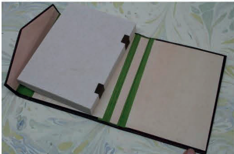
Fig. 210. A model of an unsewn textblock with connective strips (of leather) and a wrapper binding.
