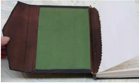
Fig. 204. A model of a full leather binding with cloth doublures on the boards, a leather doublure on the flaps, and an additional leather inner joint. The leather turn-ins overlap the cloth.
