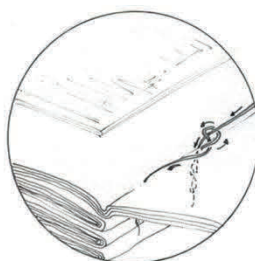
Fig. 39. Drawing of the knotted thread. The knot is formed after the thread linked on the spine and was taken back in the gathering.
