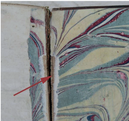
Fig. 61. Or. 755 (1612). Damage in the joint of the marbled paper doublure with stub reveals the cloth flange underneath. As the inner joint is completely torn, it may not be immediately clear that this cloth is the extension of the spine-lining. The arrow points at the cloth. The cloth pattern, visible on the left side of the joint, is only an imprint of the cloth in the paste-layer on the torn paper.
