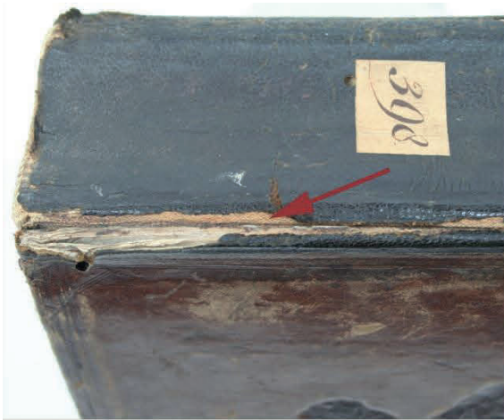
Fig. 63. Or. 398 (1571). The textile spine-lining is cut and used on the bias. The damage to the leather joints gives visual access to the spine-lining; the arrow points at the threads of this cloth.
