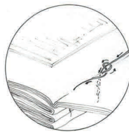
Fig. 39. Drawing of the knotted stab stitch. The knot is formed after the thread linked on the spine and was taken back in the gathering.
