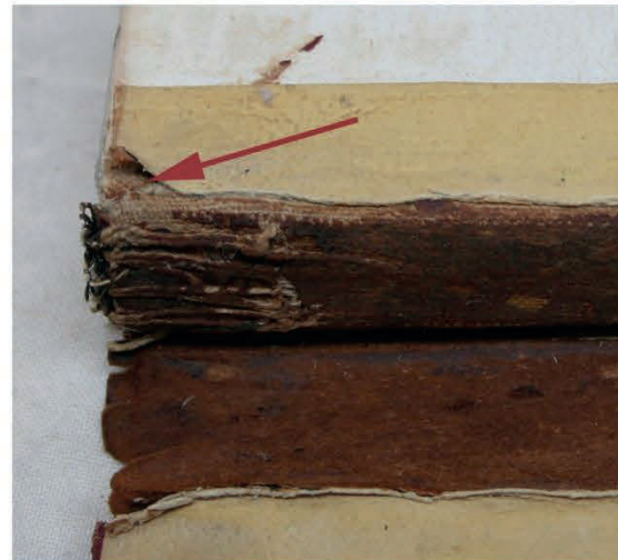
Fig. 62. Or. 2686 (1844). The extension of the cloth lining was adhered onto the outer leaves of the textblock; it did not function in the board attachment structure. Now that the adhesive with which the leather was pasted onto the textblock spine has lost its strength, the paper joint has split. The remaining stub covers the cloth pasted onto the textblock's outer leaf.
