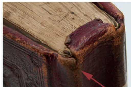
Fig. 74. Or. 10.783 (1869). The tab was moulded over the endband and slightly indented with a tool along the endband's edge. When the incision was made that allows the making of the turn-ins over the board edges, the leather was cut a little too deep.
