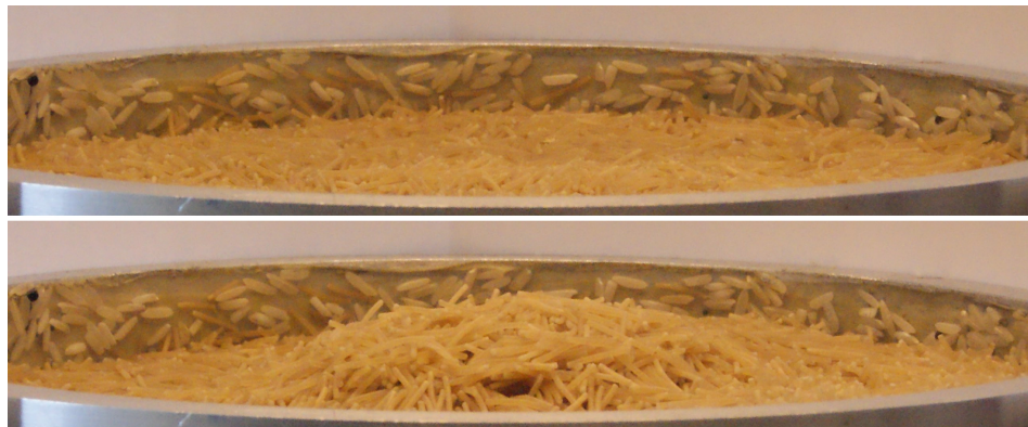
FIGURE 6.1: (top) The initial flat surface. (bottom) A vermicelli heap that has grown while we sheared the system.
