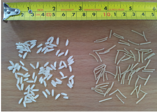
FIGURE 6.5: A picture of the particles that are used for most of the experiment: long grain “Surinam Rice” (left) and vermicelli (right).
