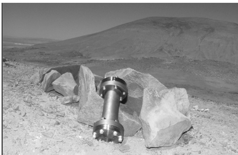
Figure 1. The sample collection site near S 24° 4' 9.6", W 69° 51' 58.1" in the Yungay region of the Atacama. Samples were collected and immediately sealed in sterile stainless steel storage containers with metal compression seals to provide a clean, hermetic transport system from the field site to the lab for analysis.
