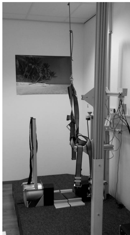
Figure 1. Experimental set-up with the Bilateral Ankle Perturbator (BAP). The participant wore a safety harness to prevent a fall and looked at a poster on the wall.
