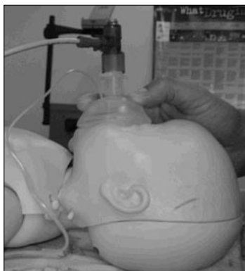
Figure 1. Placement of the open face mask demonstrated on a mannequin. The facemask was applied to the face, enclosing the mouth and nose. To ensure that there was no mask leak a finger was applied around the infant's chin was held firmly during the recording. A hot wire anemometer was attached proximally to the Laerdal mask. A bias flow of 2 L/min of air was given through the face mask.
