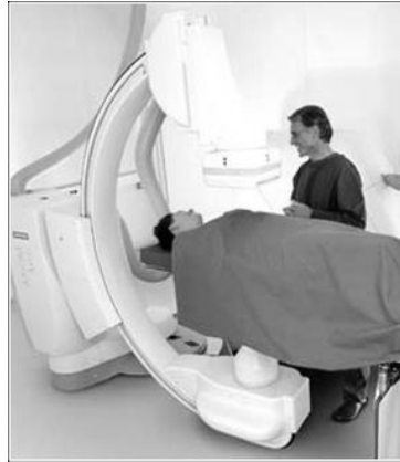
Figure 1.3: Modern X-ray system with a source on one side and a detector on the other side of the patient, both mounted on a so-called c-arm.
