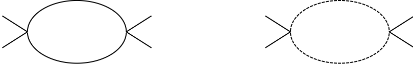
Figure 4.12: One-loop diagrams contributing to the first order correction of \beta_1 . The solid lines represent the \psi fields, and the dashed lines represent the \phi fields. The external lines are slow modes, and the internal lines are fast modes.
