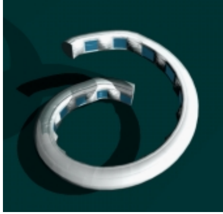
Figure 5.4: Model representation of the new Clarion HiFocus electrode, which has 16 rectangular surface contacts, located at the modiolar side of a silastic carrier. It is intended to be displaced to the modiolar wall of the scala tympani by a positioner, which is introduced separately along the outer curvature. The size of the contacts is 0.4 \times 0.5 mm for the human and 0.18 \times 0.23 mm for the guinea pig model.)
