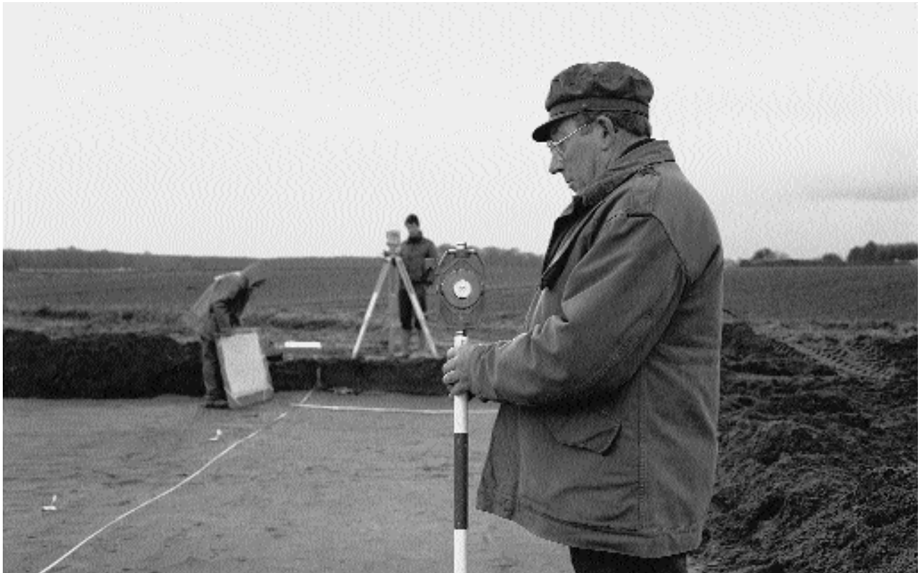
Fig. 4.10 Recording the finds and traces with the aid of an infrared theodolite.
