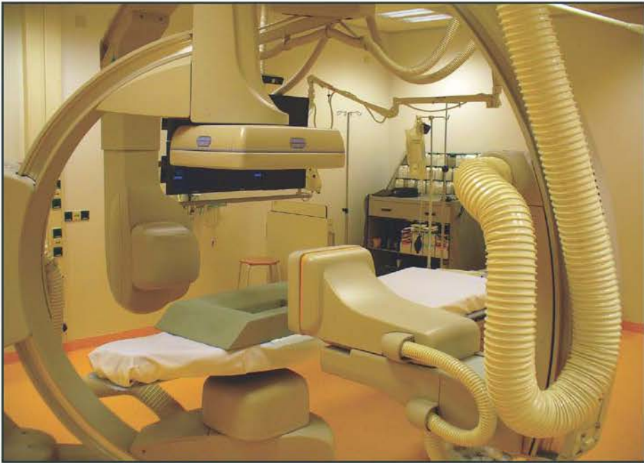
Figure 1. Bi-plane fluoroscopy set-up. Important advantage of this system is the possibility of direct manipulation of the position of the x-ray tubes by the specialist performing the intervention using the sterile dressed control panel.
