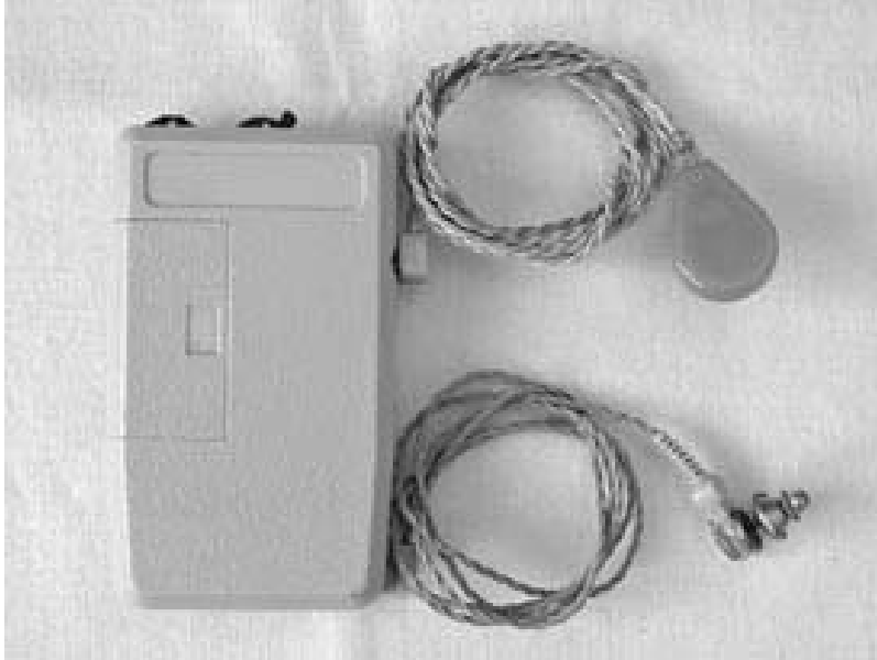
Figure 3. The single-electrode 3M/House implant (1980); measuring 8.6 cm x 5.1 cm x 1.6 cm. This was the first cochlear implant approved by the FDA. It used a transmitter that had been worn just behind the ear, a microphone that had been pinned to the clothing and a body worn single channel speech processor.
