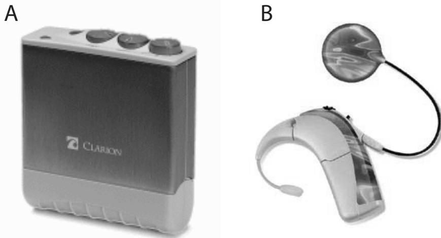
**Figure 7.** (A) Clarion CI device (1996); (B) Harmony processor (2010). Both are processors from Advanced Bionics®, where (A) is their first processor, body worn and (B) is the most recent processor, worn behind the ear.
