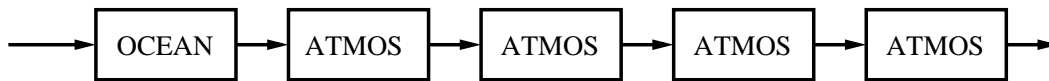
Figure 5.2: Sequential execution of the ocean and atmosphere steps for the Quasi-Geostrophic Dynamics model.
