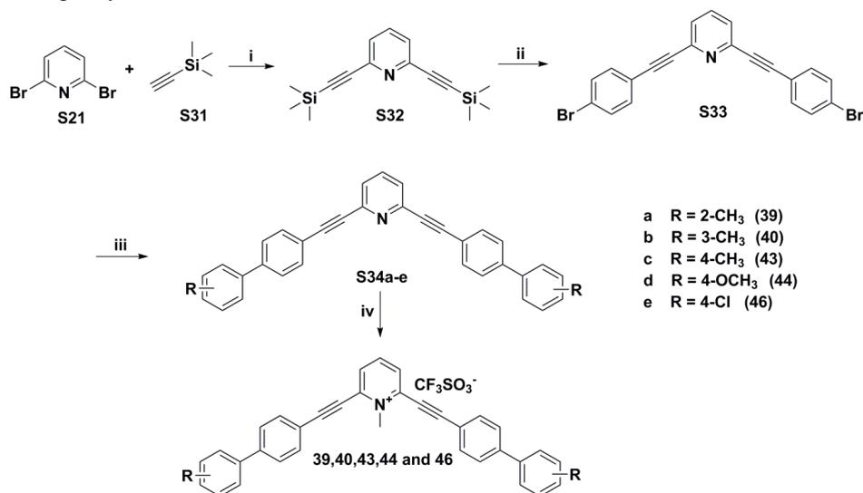
**A)** Synthesis of compounds **39**, **40**, **43**, **44** and **46**: i)  $\text{Pd}(\text{PPh}_3)_4$ , CuI, diisopropylamine, toluene, r.t.; ii)  $\text{CuCl}$ ,  $\text{PPh}_3$ , potassium benzoate, 1-bromo-4-iodobenzene, DMI,  $120^\circ\text{C}$ ; iii)  $\text{Pd}(\text{PPh}_3)_4$ ,  $\text{K}_2\text{CO}_3$ , toluene, ethanol, substituted-phenylboronic acid,  $50^\circ\text{C}$ ; iv)  $\text{CF}_3\text{SO}_2\text{OCH}_3$ ,  $\text{CH}_2\text{Cl}_2$ ,  $0^\circ\text{C}$  to r.t.
