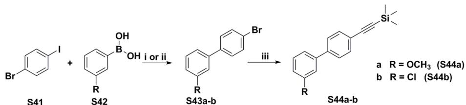
**A)** Synthesis of compounds **S44a-b**: i) 2M K<sub>2</sub>CO<sub>3</sub>, Pd(PPh<sub>3</sub>)<sub>4</sub>, toluene, ethanol, 80 °C; ii) 2M K<sub>2</sub>CO<sub>3</sub>, Pd(OAc)<sub>2</sub>, PPh<sub>3</sub>, toluene, ethanol, 80 °C; iii) PdCl<sub>2</sub>(PPh<sub>3</sub>)<sub>2</sub>, CuI, PPh<sub>3</sub>, THF, piperidine, 120 °C.
