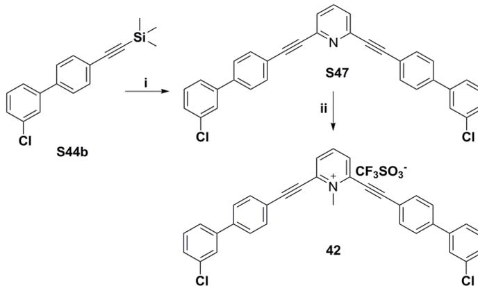
**C)** Synthesis of compound **42**: i) CuCl,  $\text{PPh}_3$ , potassium benzoate, 2, 6-dibromo-pyridine, DMI, 120 °C; ii)  $\text{CF}_3\text{SO}_2\text{OCH}_3$ ,  $\text{CH}_2\text{Cl}_2$ , 0 °C to r.t.
