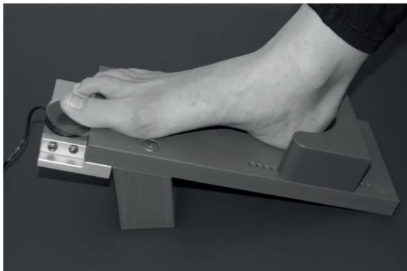
Figure S5.1: Device used for measuring toe plantar flexion force.
