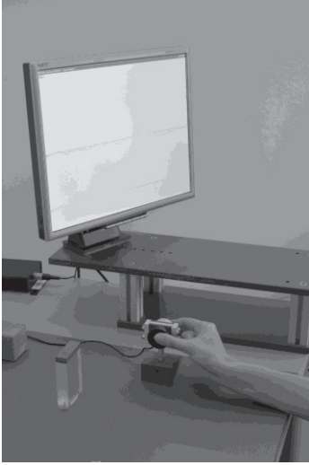
Figure 5.1: Overview of the experimental setup. Thumb force was measured during precision grip using the ‘Q-Motor’ grip instrument (Reilmann et al., 2010). Target force and real-time visual feedback of the participant’s force output were presented on a computer screen during the VF phase.
