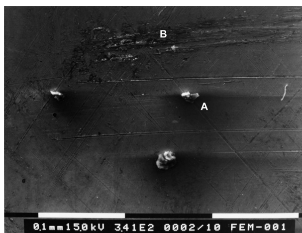
Figure 5. Scanning electron micrograph detail of a retrieved femoral component showing abrasive-adhesive wear (A) scratching and wear residue (B).
