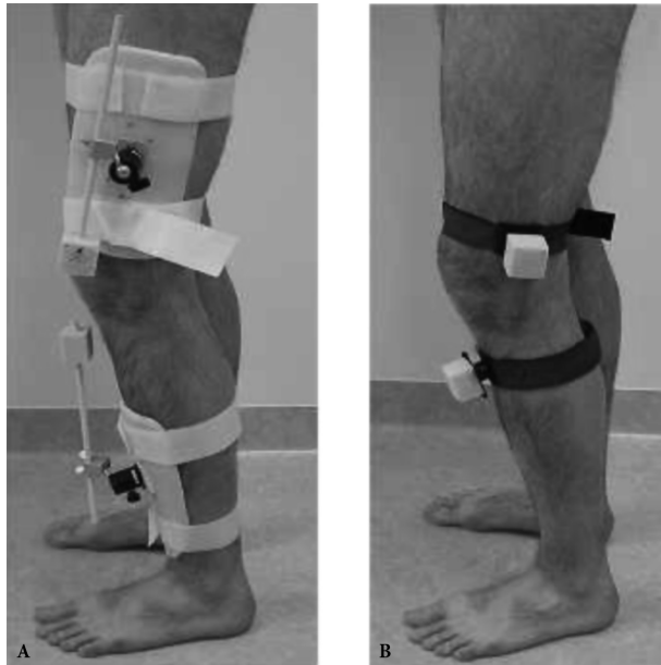
Figure 1. The plate mounted markers configuration with adjustable extensions for visualisation (A). Strap mounted marker configurations in the polystyrene blocs (B).
