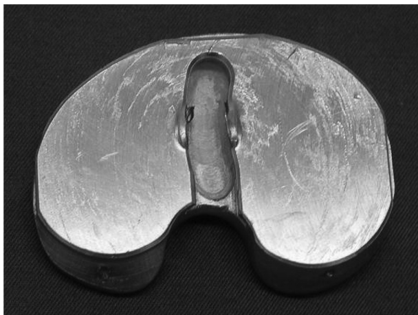
Figure 8A. Photo of the back surface of a retrieved mobile bearing tibial insert showing a rotating striation.
