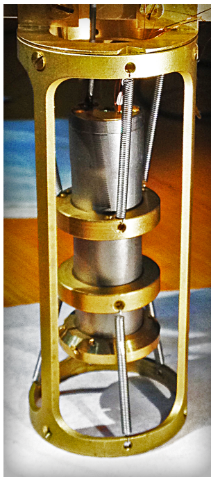
Figure 5.1: By suspending the experiment (housed in the Nb tube) in a frame with some soft springs, external vibrations are mitigated.
