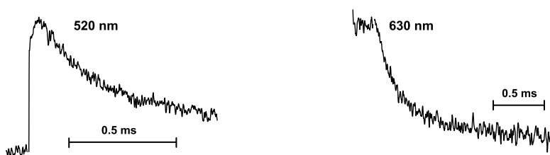
Fig. 4.6. Transient absorbance changes showing the rapid formation and further slower decay of 5-dRf semiquinone radical measured at 520 nm (upper trace), and reduction of Cu(II) azurin measured at 630 nm (lower trace). The concentration of Im-Cu-H117G azurin was 25 \mu\text{M} , in 20 mM MES pH 6 and 100 \mu\text{M} 5-dRf at room temperature.
