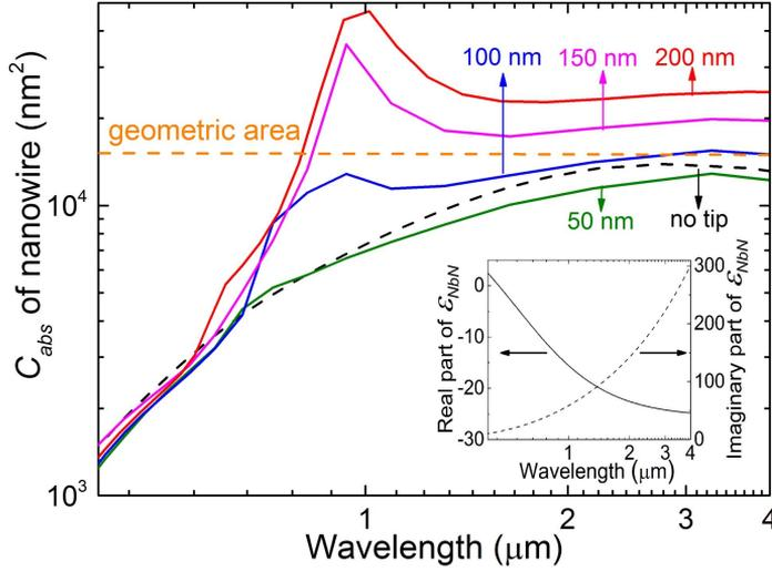
Figure 7.3: Calculated absorption cross section  $C_{abs}$  of the nanowire as a function of wavelength in the presence of a tip of varying length. The black dashed line is the absorption of the nanowire without tip and the colored curves are with tips of different lengths from 50 nm to 200 nm. As a reference, the horizontal dashed line shows the geometry area of the  $100 \times 150 \text{ nm}^2$  nanowire. The real and imaginary parts of the relative permittivity of NbN are shown in the inset.
