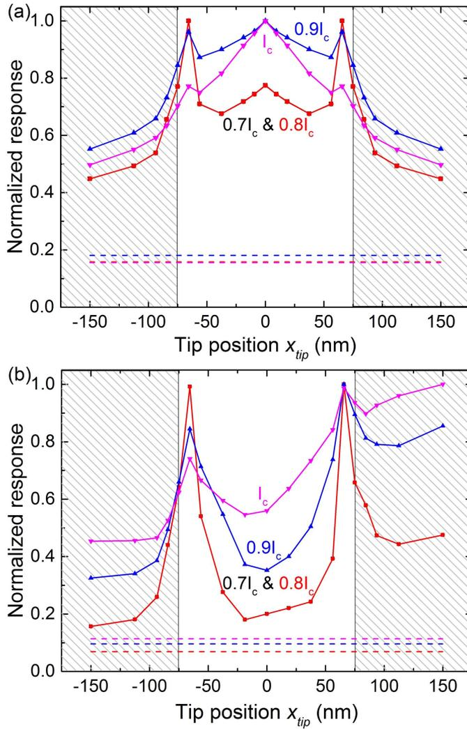
Figure 7.7: Detector response as a function of tip position  $x_{tip}$  for light incident from (a) the  $y$ -direction and (b) the  $x$ -direction. The unshaded area corresponds to the nanowire. The calculation uses the local detection efficiency  $LDE(x, I_b)$  in Fig. 7.6 at several bias currents. The dashed lines (background signal) are the detector response without tip in the system. Each curve is normalized to its maximum value to compare the shape of the response.
