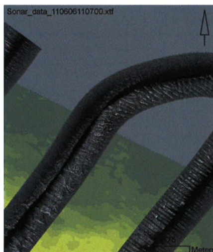
Figure 10. Detail of the sonar images taken on Monday, June 6, 2011. Visible to the north is the intact seafloor (no bathymetric data available). The section on which bathymetric data are available (marked in shades of yellow and blue) shows the disturbance on the slopes of the extraction zone.
