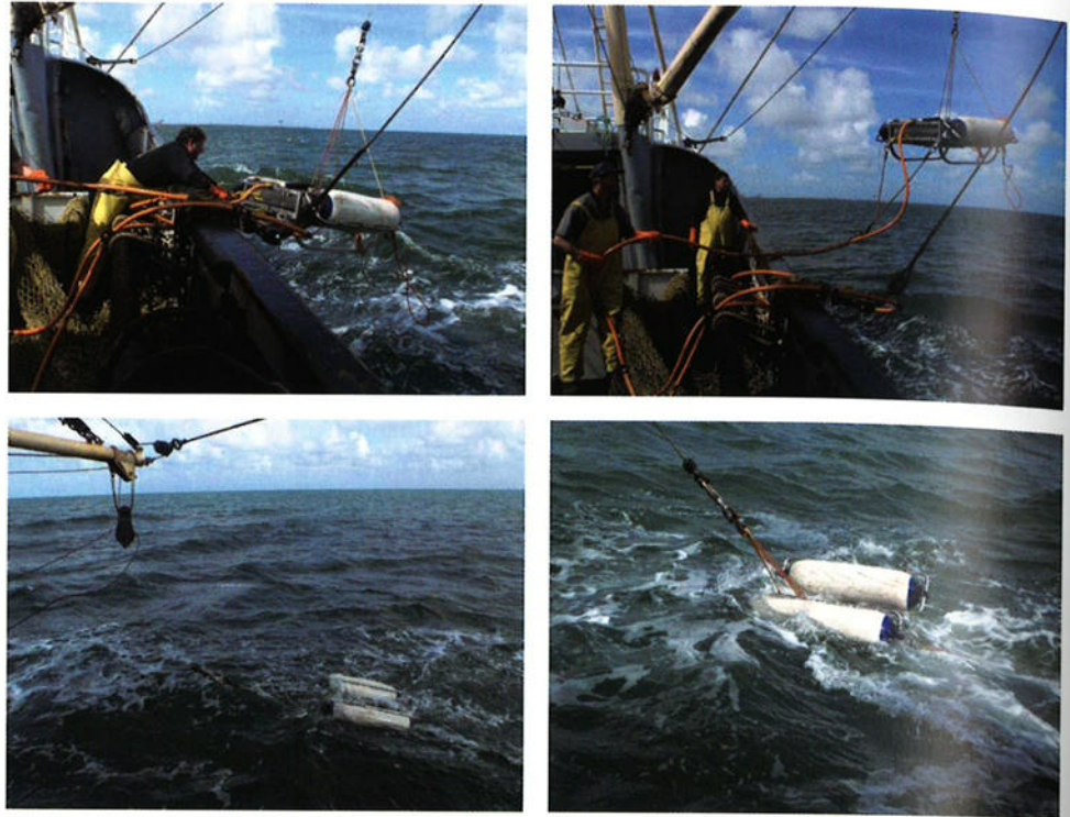
Figure 3. Launching the Boomer from the trawler's starboard side. Photos: Wiersma and Mesdag 2013, 5.
