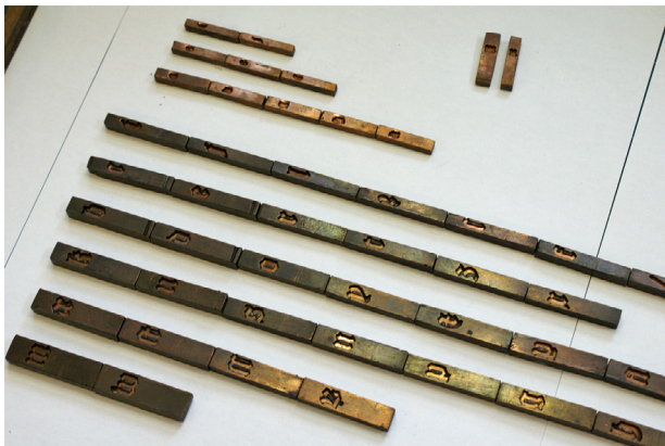
Figure 7.12 Van den Keere's matrices for Canon Flamande and Parangonne Flamande in rows.
