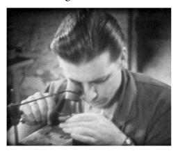
As the name of the profession reveals, the punchcutter cut punches. In the period from 1450 until 1500, the complete typefounding process, which included the cutting of punches, the striking and justification of matrices, and the casting of type, was the work of a single person. In later times these activities were also split
