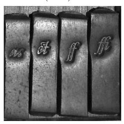
These are matrices that have been struck with a punch and are unjustified, which means that they have not been further prepared for the production of type. Due to the force required to obtain a proper impression of the image of the letter on top of the punch into the piece of copper, the latter is distorted. Matrices were traded both raw and justified.
