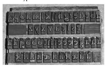
This term comprises the forms of type that find their origin in the system Gutenberg developed for typesetting and printing with separated letters. Gutenberg placed letters onto rectangles and, irrespective of their sequence, the spacing of these letters was uniform.
