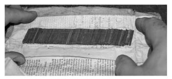
These were collections of pre-cast type that were delivered together with matrices in case the matrices were not justified for casting with fixed registers. The caster could use these by putting a pre-cast letter into the related matrix and then enclosing it with the mould's registers. Consequently the caster did not have to check the spacing/fitting.
