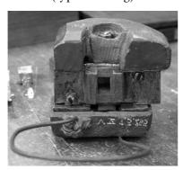
This is a hand-held device for the casting of foundry type. The Dutch term 'gietfles', which literally translated means 'pouring bottle' exactly describes what it is. A typefounder's mould consists of two parts that are kept together by the caster's hand. The halves can be slid in one direction to control the width of the shank, of which the aperture can be seen in the centre of the mould in the image above. At the end of the shank the matrix is fixed with a large and easy to remove
