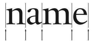
These are the vertical boundaries that mark the character widths. In contrast with digital type, side bearings in movable type are physically present as the edges of the metal rectangles on which the letters are placed.
