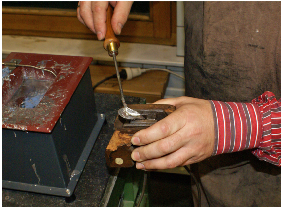
Figure 6.6 Molten lead is poured into the shank.
