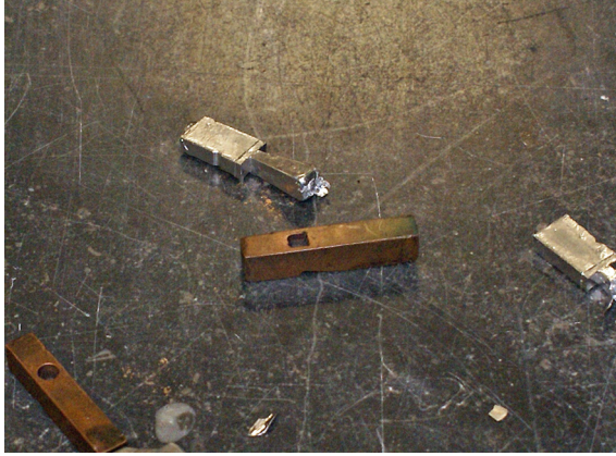
Figure 6.8 The tang is a wedge-shaped tail.
