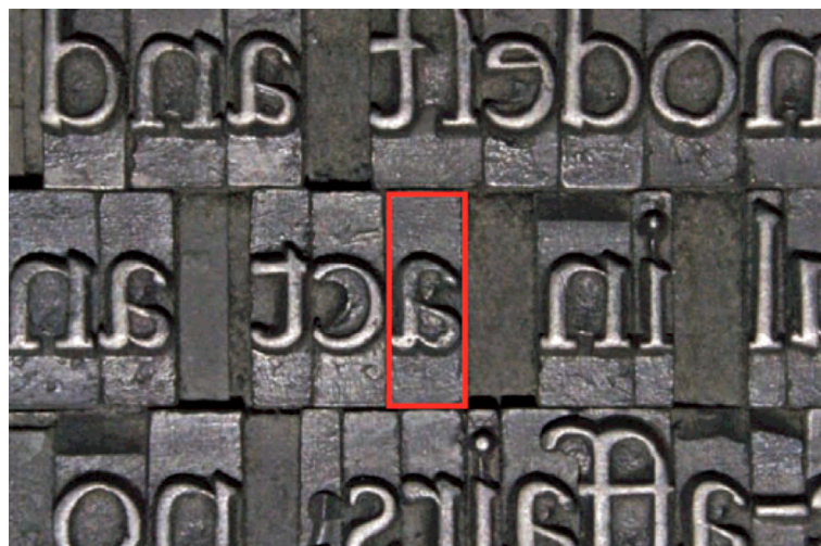
Figure 1.8 For movable type the letters and their surrounding space were captured in rectangles.
