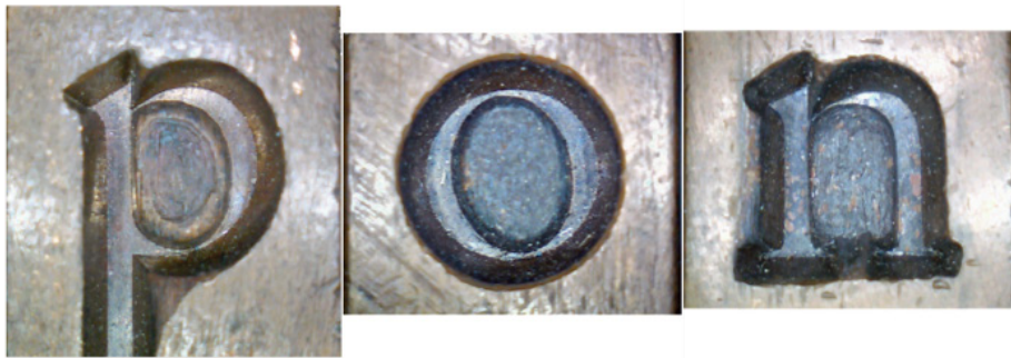
Figure 7.10 Word typeset in Gros Canon Romain matrices.
