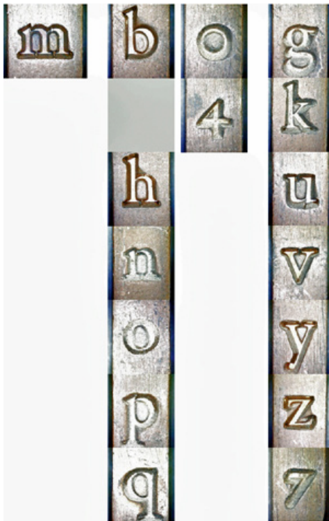
Figure 9.2 Ascendonica Romain matrices of the MA7 set showing standardised widths. 225
