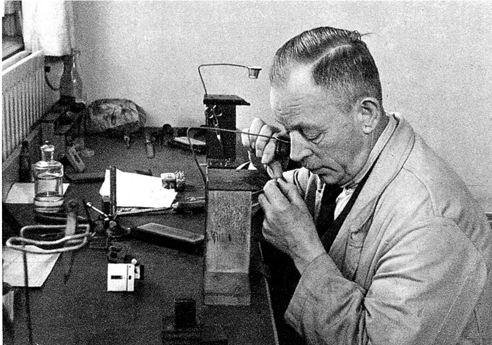
Figure A5.8 Rädisch cutting punches at Joh. Enschedé en Zonen in 1951. 363
