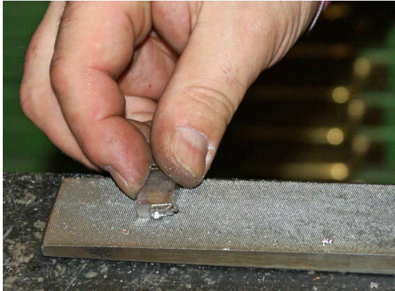
Figure 6.9 The rough edges are filed.
