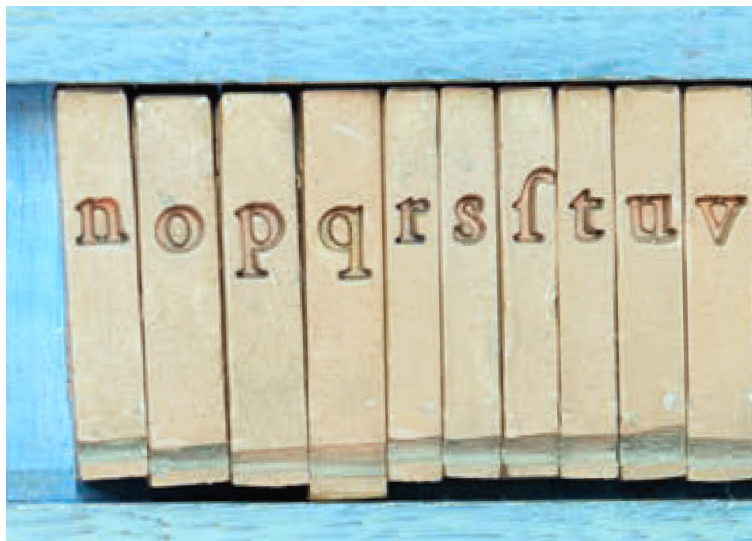
Figure 9.4 Ascendonica Romain matrices of the MA8 set showing different widths.
