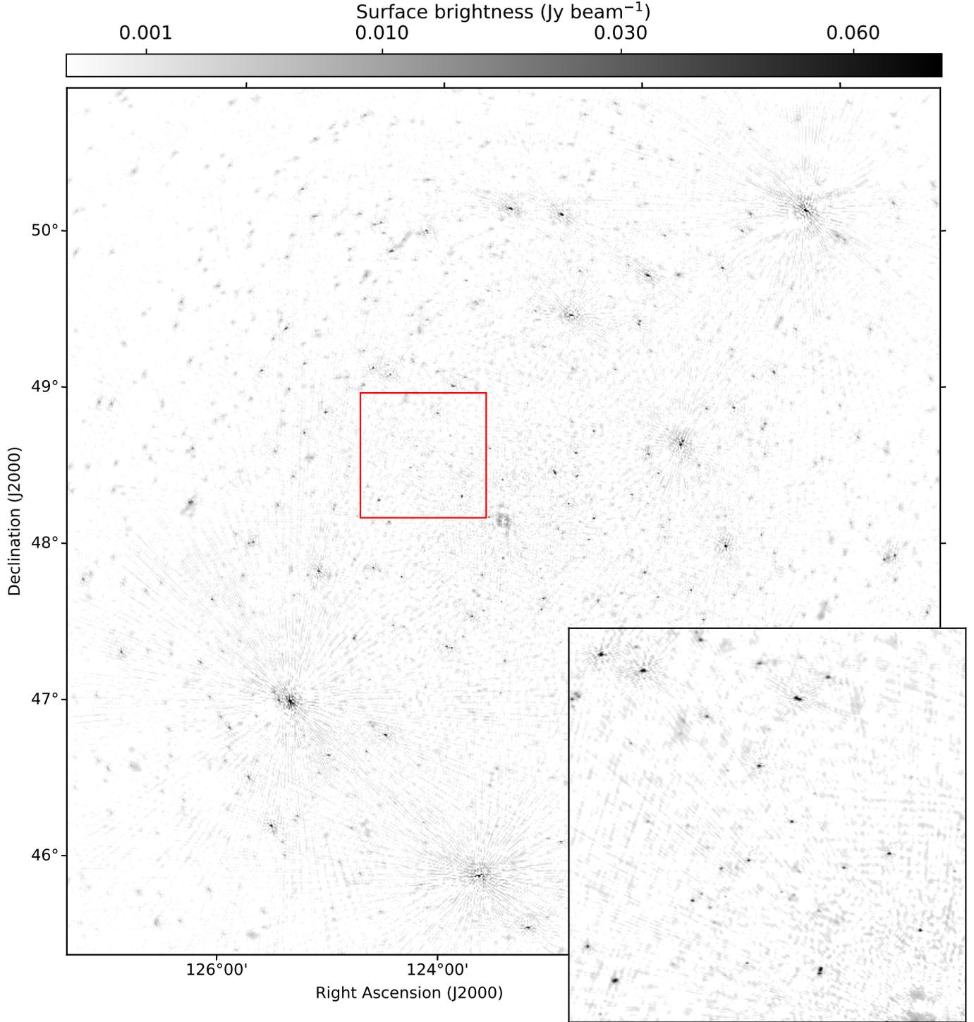
**Fig. 9.** Image of the field around 3C 196 (subtracted) at 152 MHz obtained with LOFAR HBA. The image resolution is  $16'' \times 10''$  and the rms noise is  $450 \mu\text{Jy beam}^{-1}$ . The red square shows the region that is zoomed-in in the bottom right corner.
