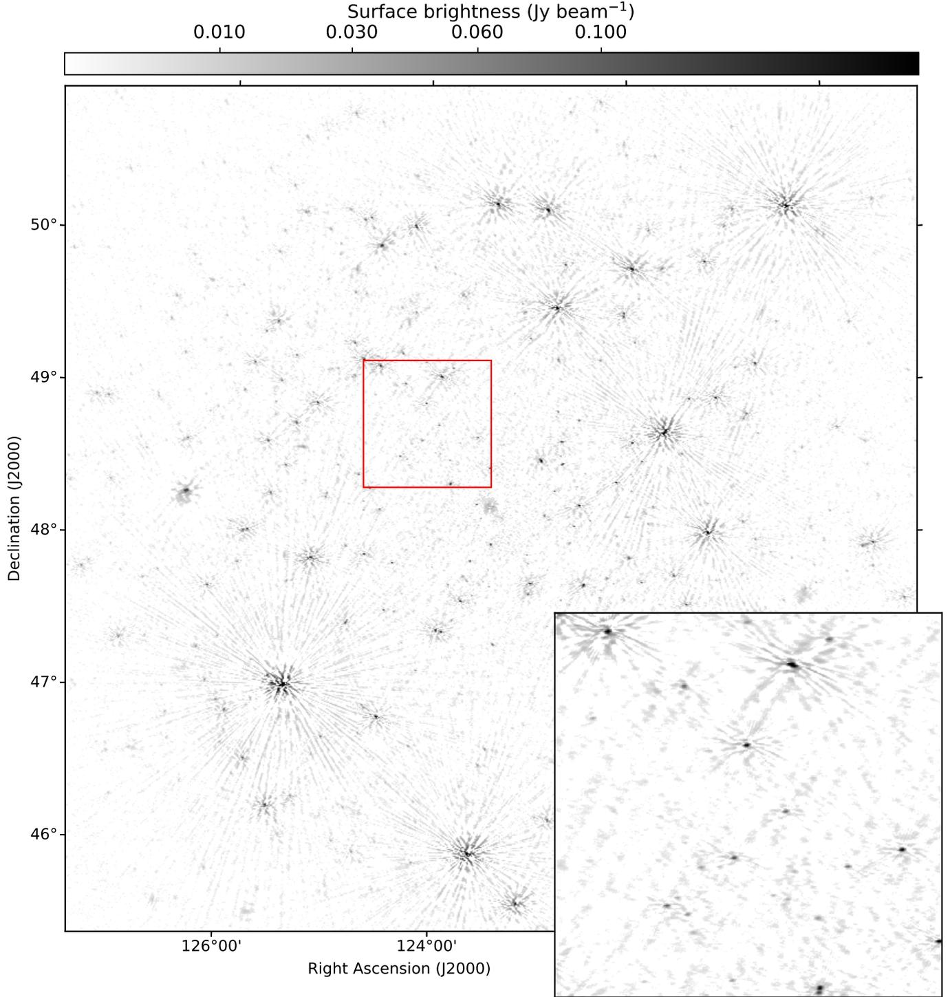
**Fig. 8.** Image of the field around 3C 196 (subtracted) at 54 MHz obtained with LOFAR LBA. The image resolution is  $26'' \times 14''$  and the rms noise is  $3 \text{ mJy beam}^{-1}$ . The red square shows the region that is zoomed-in in the bottom right corner.
