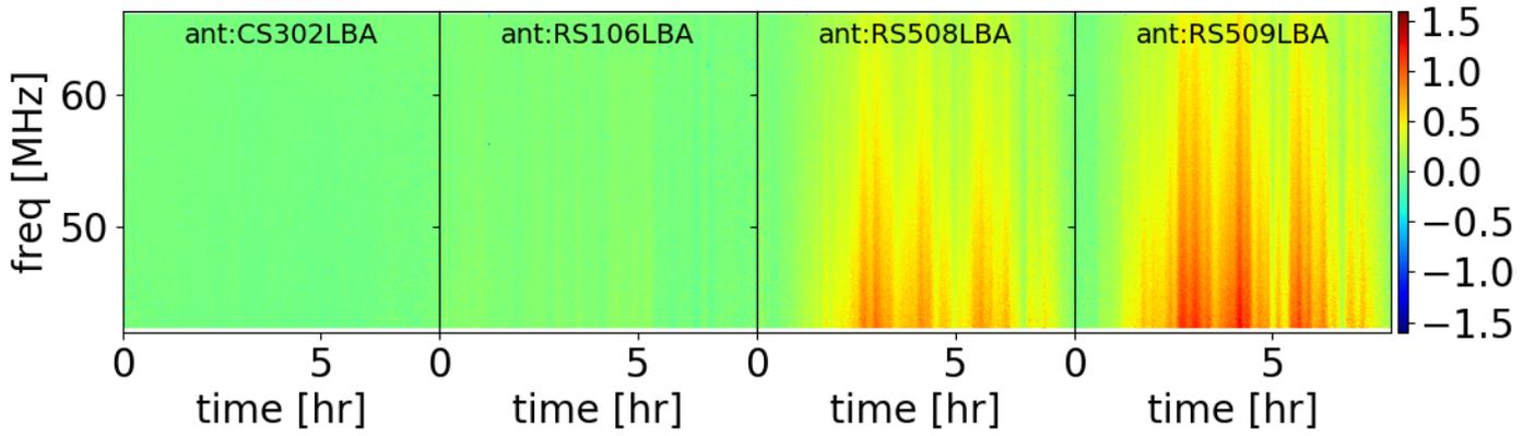
**Fig. 4.** Same as Fig. 3 but is the rotation angle in radians of the Jones rotation matrix is colour coded. The two most RSs show clear evidence of Faraday rotation. The two stations are close in location, therefore the effect is similar. The HBA equivalent is shown in Fig. A.2.
