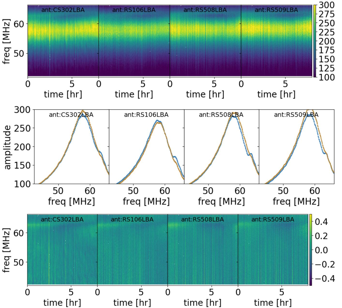
**Fig. 6.** Same as Fig. 3. *Top panel:* amplitude solutions for the XX element of the diagonal matrix. *Mid-panel:* time median of the amplitude solutions; this represents the instrument bandpass. Blue is for the XX polarisation and brown for the YY. *Bottom panel:* residuals after dividing the top panel by the time-independent bandpass. The HBA equivalent is shown in Fig. A.4.
