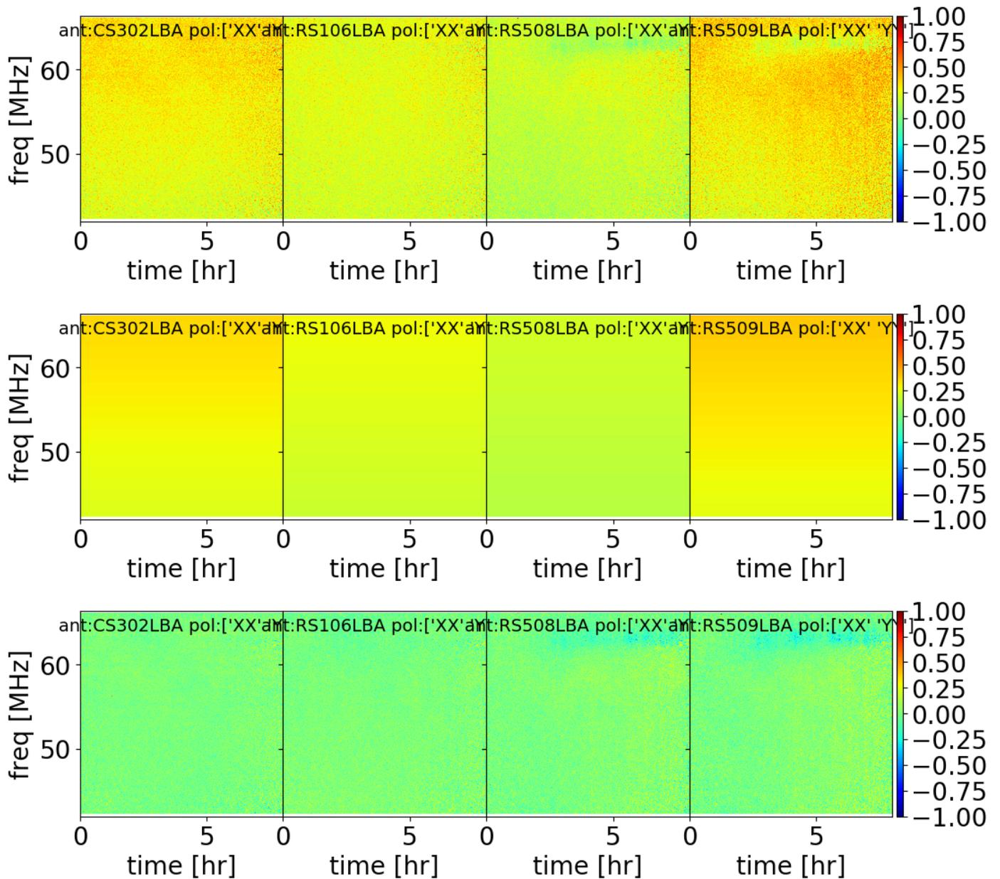
**Fig. 5.** Same as Fig. 3. *Top panel:* differential (XX-YY) phase solutions. *Mid-panel:* the time-independent delay fit performed by LoSoTo. *Bottom panel:* differential phase solutions after the subtraction of the delay. The HBA equivalent is shown in Fig. A.3.
