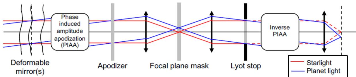
Figure 2. General coronagraph layout (adapted from Ruane et al, 2018). The schematic shows a coronagraph with one or more deformable mirrors, optics for phase induced amplitude apodization (PIAA), a pupil-plane apodizer mask, an image plane mask, a Lyot stop, and inverse PIAA optics. Modern coronagraph designs employ various combinations of these planes.
