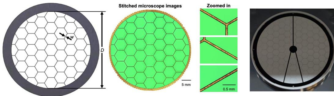
Figure 6. Segmented pupil masks manufactured for (*Left*) the Decadal Survey Testbed using the off-axis LUVOIR-B aperture. The mask diameter is  $D = 41.75$  mm and the gap width,  $w$ , of 50-100  $\mu\text{m}$ . (*Right*) the PIAACMC testbed using the on-axis LUVOIR-A aperture with  $D = 43$ mm and gap width of 20  $\mu\text{m}$ .
