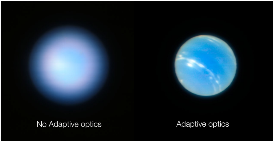
Figure 1.4: Observations of Neptune with the new Narrow Field Mode of MUSE with AO correction provided by the LTAO system. The LTAO shows almost diffraction-limited performance. Image credits to ESO/P. Weilbacher (AIP).
