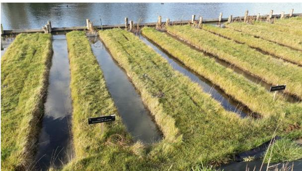
**Fig. 2.** Photographic overview of the experimental site 'the Living Lab'. Top to bottom: adjoining reservoir, wave barrier, macrophytes, netting, experimental ditches.
